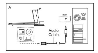
B. Plug one end of the audio cable into the jack on the front of the treadmill near the power cord. Plug the other end of the cable into a 3.5mm Y-adaptor (available at electronics stores). Plug the Y-adaptor into the PHONES jack on your computer. Plug your headphones or speakers into the other side of the Y-adaptor.
